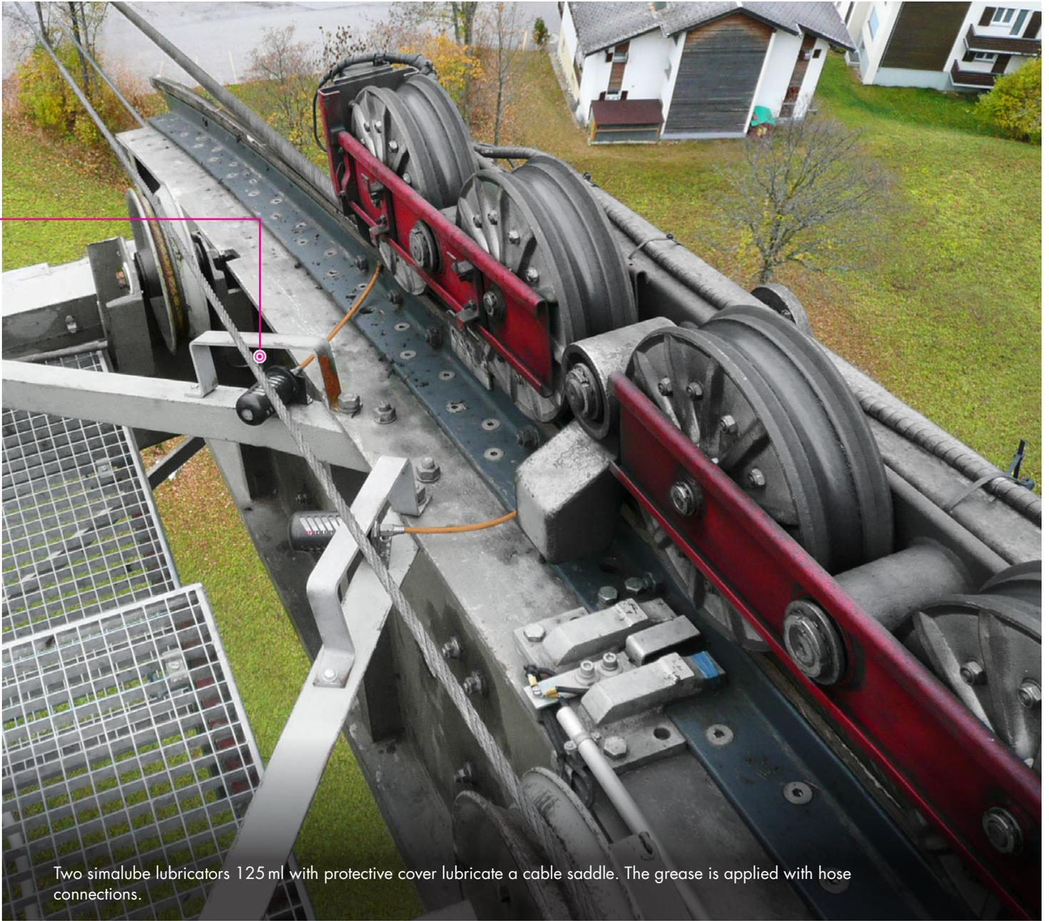
Two simalube lubricators 125 ml with protective cover lubricate a cable saddle. The grease is applied with hose connections.
