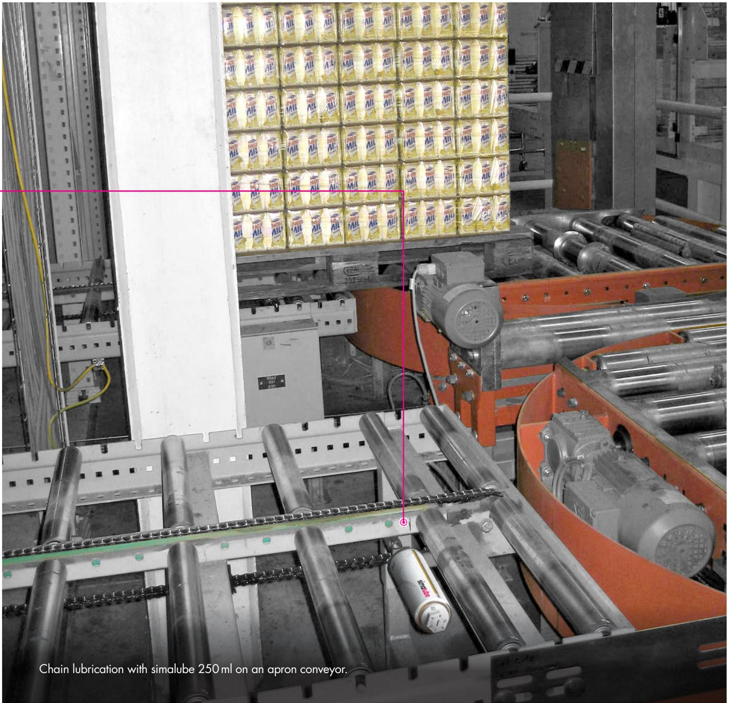
Chain lubrication with simalube 250 ml on an apron conveyor.
