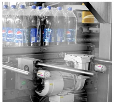
The bearing on the gear box is lubricated with two 60 ml simalube lubricators.
