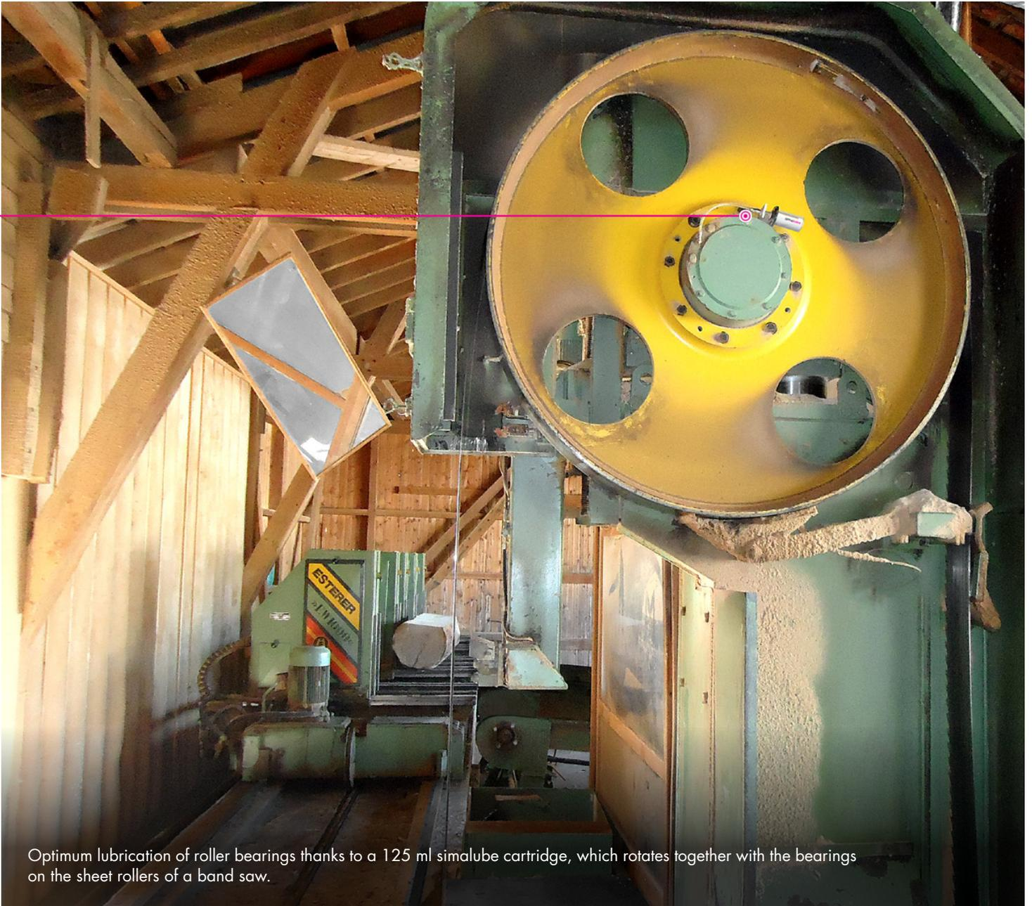
Optimum lubrication of roller bearings thanks to a 125 ml simalube cartridge, which rotates together with the bearings on the sheet rollers of a band saw.
