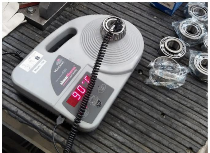
The portable VOLCANO IH 025 is used for the installation of gear shafts. For this purpose, a tapered roller bearing is heated to the desired temperature using the temperature monitoring system.
