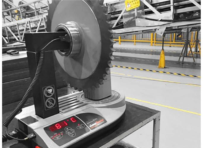
The induction heater IH 070 is the ideal choice for heating the return sprocket of the step chain of an escalator.
