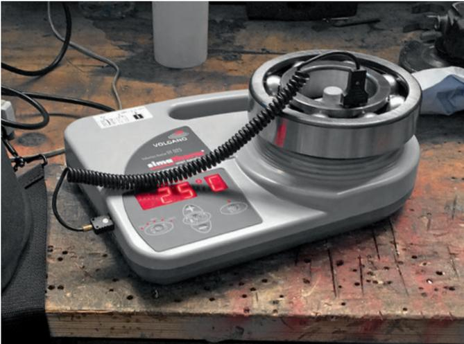
The portable VOLCANO IH 025 weighs only 3.5 kg but can easily heat parts weighing up to 10 kg to 110°C.
