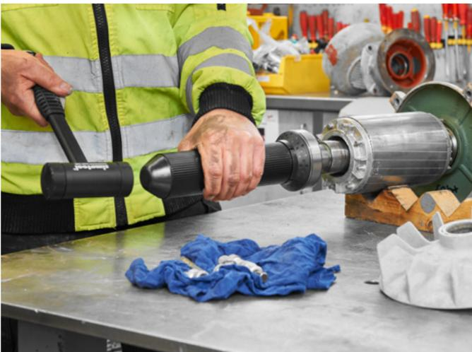
The Fitting Tool FT 33 ensures that the mounting force is evenly distributed across the inner and outer rings of the bearing and therefore does not stress the rolling elements.
