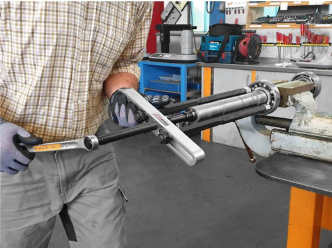
With the aid of extensions, the BP 160 dismounting tool kit also makes it possible to dismount hard-to-reach bearings easily and professionally.
