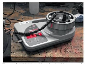
The portable VOLCANO IH 025 weighs only  $3.5\,\mathrm{kg}$  but can easily heat parts weighing up to  $10\,\mathrm{kg}$  to  $110^\circ\mathrm{C}$ .
