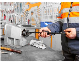
Knowhow: using a Seal Puller SP 50 to remove a radial seal from a gearbox without damaging the housing or shaft.
