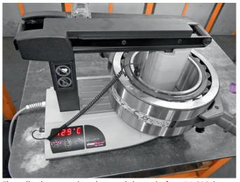
The roller bearing placed around the coil of an IH 210 heater is heated by induction. A simatool Bearing Handling Tool is in place to position the bearing on the shaft, once the specified mounting temperature is reached.
