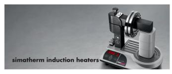
The best way to avoid unwanted stresses when assembling interference-fit parts is to heat the outer part just enough to produce a temporary clearance. simatherm induction heaters allow this to be done precisely, evenly, quickly and efficiently. Other methods of heating are slower, less controlled and can cause more harm than good to bearings.
