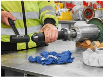
The Fitting Tool FT 33 ensures that the mounting force is evenly distributed across the inner and outer rings of the bearing and therefore does not stress the rolling elements.
