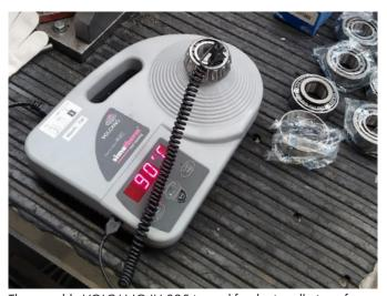
The portable VOLCANO IH 025 is used for the installation of gear shafts. For this purpose, a tapered roller bearing is heated to the desired temperature using the temperate monitoring system.
