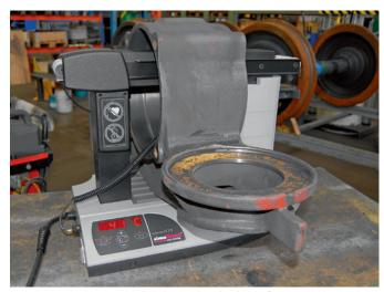
Working on a train wheel-set, the high-performance induction heater IH 210 heats a massive bearing housing to allow a bearing to be inserted.
