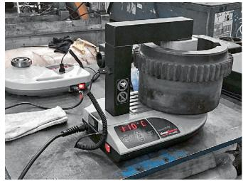
The simatherm induction heaters VOLCANO IH 025 and IH 070 with two differently sized workpieces: the model IH 070 (in the front) heats a gearwheel sleeve to the specified installation temperature.
