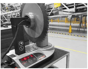
The induction heater IH 070 is the ideal choice for heating the return sprocket of the step chain of an escalator.
