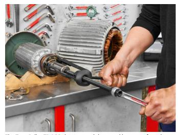
The Twin Puller TP 150 does it: a tightly seated bearing of an electric motor is removed without risking damage to the housing or the shaft.
