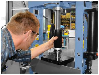
The FT-P is the ideal solution for installations with greater forces, as the tool can be used on a press. High-quality aluminum rings that do not deform even with press-in forces of 5 tons.
