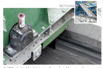
A 125 ml simalube lubricates the pedestal bearing of a conveyor belt.
