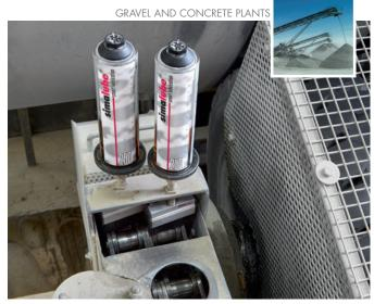
Two 250 ml simalube lubricators with brushes lubricate and clean the chain drive of a drum washing machine.
