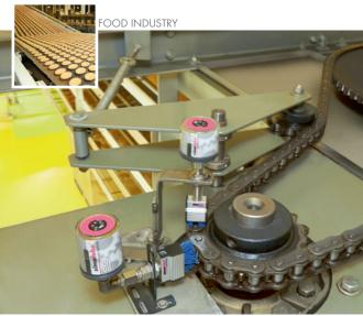
The drive chain of a transport belt, which allows rolls to cool, is cleaned with special blue brushes and lubricated with 2 simulube  $\,$  SL18 in 30 and 60 ml sizes.
