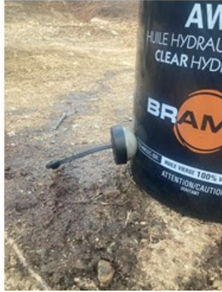
Rupture Seal Environmental emergency response test with water in a bucket on Nobles Resources Inc. operations.
