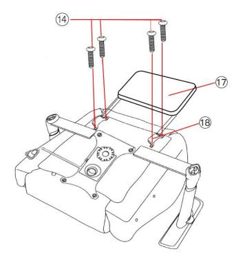
\* ① Screws have been assembled on the seat, please loosen them for further assembly.\*
