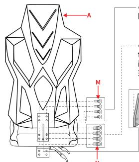
•Align the steel plate with the four holes on the backrest and screw in the 4 screws.
