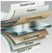
Steel skins are protected through a tough, layered coating system, including a hot-dipped galvanized layer, a protective metal oxide pretreatment and a baked-on primer and top coat.
