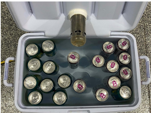
Figure 5. A water bath consisting of a cooler and sous vide device worked used as a stand-in for small-batch pasteurizers.
