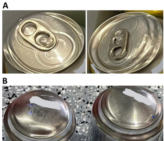
Figure 6. Visual deformation (buckling) of the can lid (A) or dome (B).
