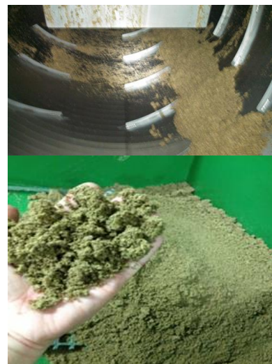
Top: screened spent hops inside of rotary drum. Bottom: spent hops after being dewatered.
