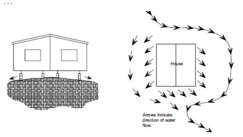
Grade the ground so that water under porches, decks, and recessed entries flows away from the home. If proper grading is not possible, use other methods such as a drain tile and automatic sump pump system to remove any water that may collect under the home.
