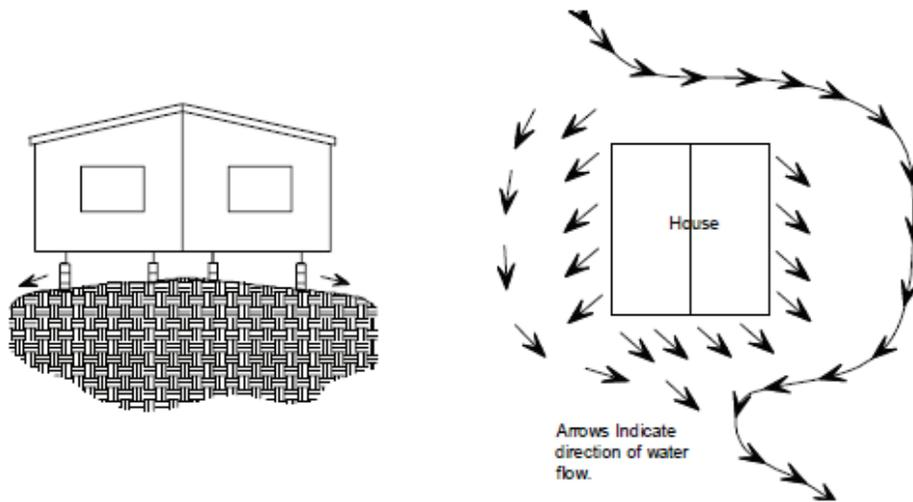
Grade the ground so that water under porches, decks, and recessed entries flows away from the home. If proper grading is not possible, use other methods such as a drain tile and automatic sump pump system to remove any water that may collect under the home.
