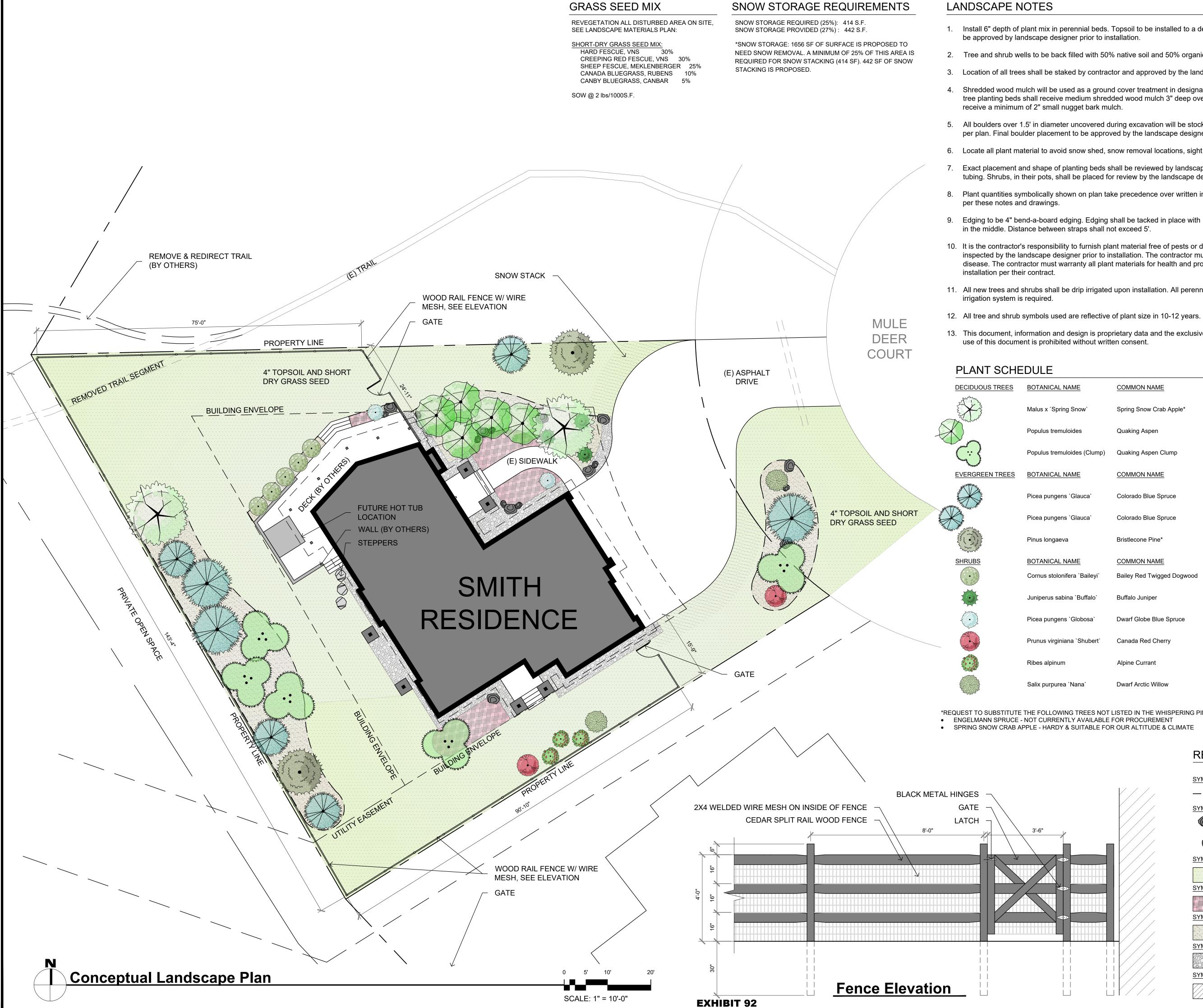
1. Install 6" depth of plant mix in perennial beds. Topsoil to be installed to a depth of 4" in all disturbed areas. All soil must
