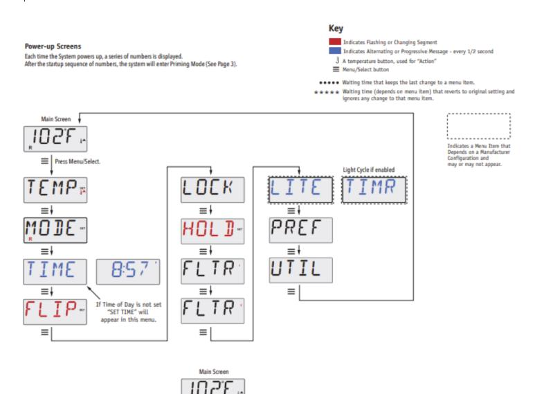
Waiting a few seconds in the Main Menu will allow the display to revert to the Main Screen. Most changes are not saved unless Menu/Select  $\equiv$  is pressed. Refer to key above.
