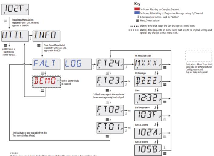
Waiting a few seconds inside the Fault Log Menu will allow the screen to return to normal operation.
