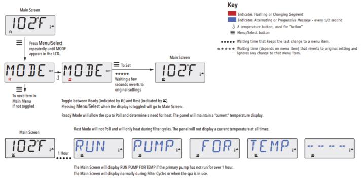
If the primary pump has been off for an hour or more, when any function button, EXCEPT Light, is pressed on the panel, the pump used in conjuncton with the heater will run so that temperature can be sensed and displayed.
