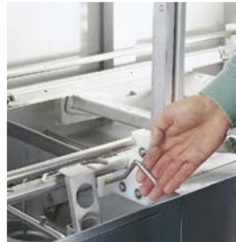
All the tanks are drained with one lever. All the bottom valves and the overflow pipe are automatically closed when the rinse section door is closed.
