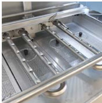
All the washing arms are identical. The arm is removed and attached by using a quick joint.
