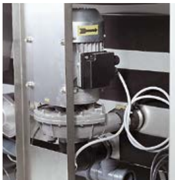
When the machine is drained, no water remains in the pumps - hygiene is improved.
