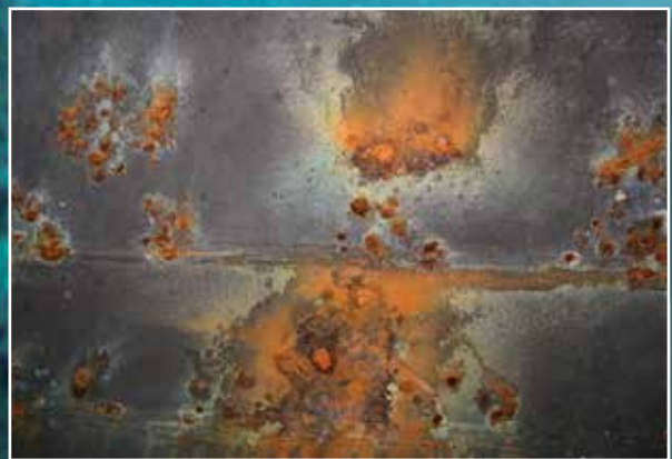
Corrosion 'blisters' on hull plate.
