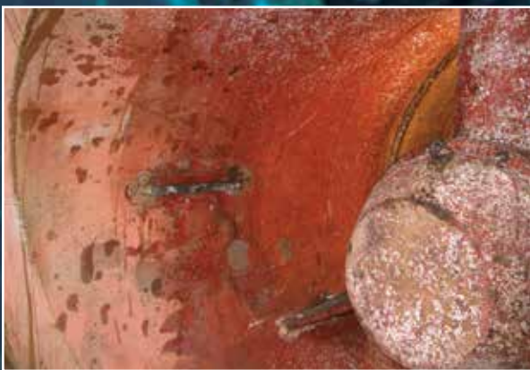
Corrosion around bow thruster.
