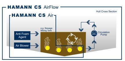
the substance of the plant, the piping and ultimately the ship's structure. Sedimentation occurs when the suspended solids settle and concentrate in the lower layers of the sewage in a tank. When the "thick" lower layers are fed into the STP/AWTS, they may cause clogging of valves, sensors and pipes of the plant. A HAMANN CS Air tank aearation system compensates
