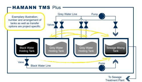
sewage is transferred to the sewage mixing tank or another holding tank. This ensures that the available tank capacities are used in the best possible way, that the filling of all tanks is optimally coordinated and that a mixture of blackwater and greywater is available in the sewage mixing tank for feeding into the STP/AWTS.
