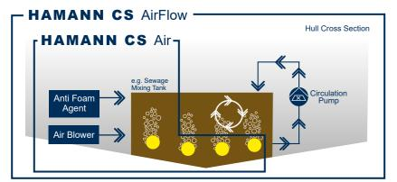
the substance of the plant, the piping and ultimately the ship's structure. Sedimentation occurs when the suspended solids settle and concentrate in the lower layers of the sewage in a tank. When the "thick" lower layers are fed into the STP/AWTS, they may cause clogging of valves, sensors and pipes of the plant. A HAMANN CS Air tank aearation system compensates the oxygen consumption by supplying fresh oxygen
