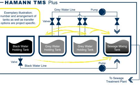
sewage is transferred to the sewage mixing tank or another holding tank. This ensures that the available tank capacities are used in the best possible way, that the filling of all tanks is optimally coordinated and that a mixture of blackwater and greywater is available in the sewage mixing tank for feeding into the STP/AWTS.
