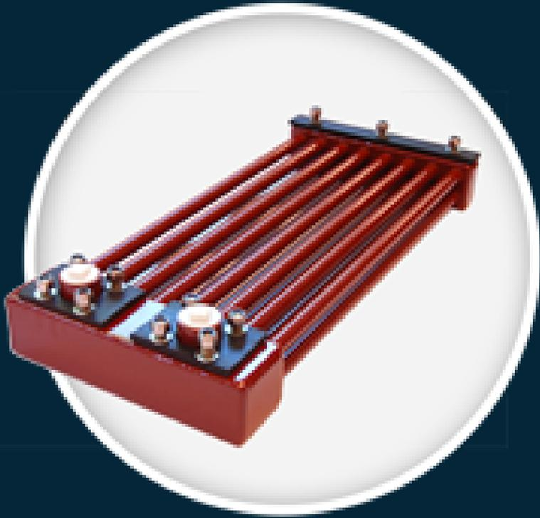
A Steel cooler is a closed-circuit cooling system mounted externally on the vessel's hull below the waterline. The concept of steel cooling is similar to the application of a radiator on a car. Engine coolant is circulated through the steel cooler, which transfers heat from the coolant before it returns to the engine. The steel cooler is in constant contact with seawater allowing the cooling system to efficiently transfer heat between the coolant and seawater
