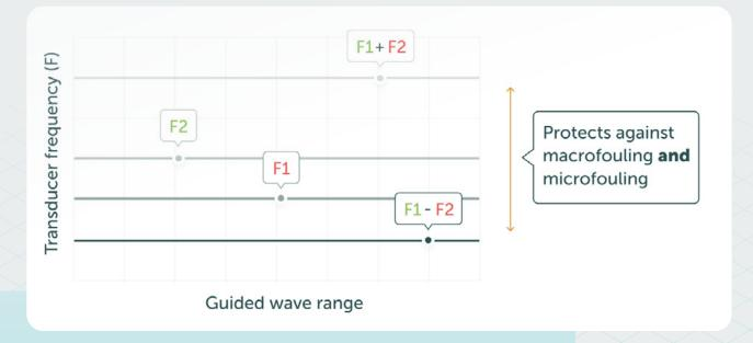
This broader spectrum disrupts a wider range of fouling organisms, making the antifouling system more versatile and effective. Additionally, the combination of Guided Wave and Heterodyning principles ensures that the energy is channeled more efficiently and over greater distances, providing superior antifouling protection compared to systems using single frequency transducers.
