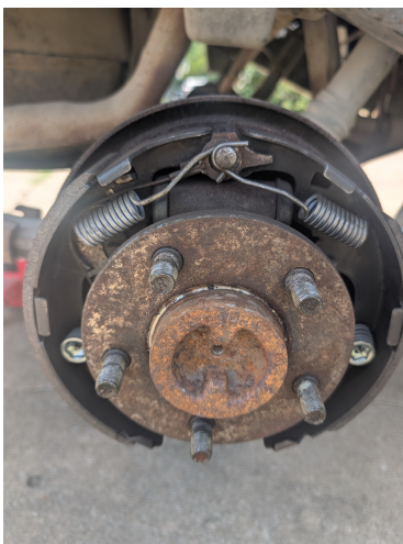
Rear brake assembly during inspection. Shoes retained substantial lining and no visible fluid contamination was found.
