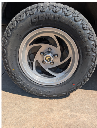
New OEM-size 215/75R15 all-terrain tire installed on the Jeep.
