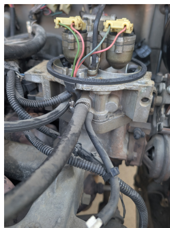
Installed Howell throttle-body injection system.
