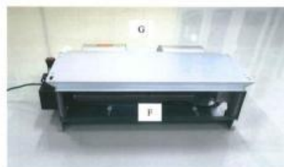
Figure 7. The distribution of two detecting points at the air inlet and outlet windows of the Edda Air ® PS-501T Plasma Ions Air Sterilizer
