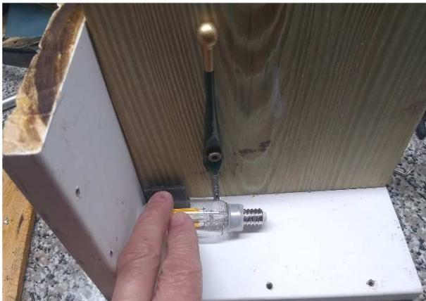
Once the bulb is well scored which may take several turns in the fixture, the glass can be separated by alternate heating and cooling. I used the hot air from a solder rework station to heat the glass and a can of cool water to cool the glass. Three cycles of heat and cooling is usually sufficient to separate the glass. A heat gun or hair dryer may be sufficient as the heat source. Some internet sources suggest using a candle.
