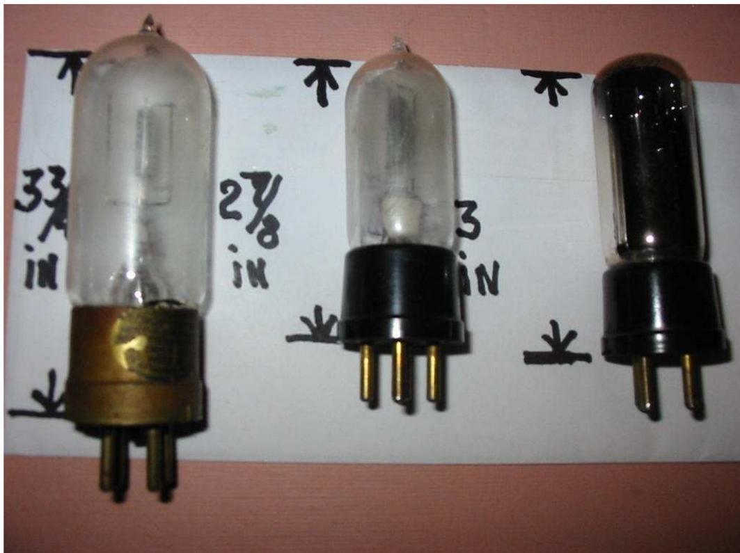
The plastic shell can be painted to look similar to the original WD11 with its silver getter. Use a good quality silver paint like Kester Chrome. Apply the paint to the outside of the shell. Paint applied to the inside of the shell will appear shiny on the inside but appear gray and dull on the outside since it is viewed from the “back side” of the paint.
