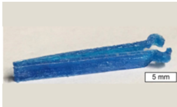
A pair of tweezers made using cellulose. An anti-bacterial die was used to make the instrument safe for use for medical purposes.
