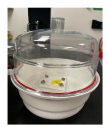
Samples placed in the vacuum desiccator
