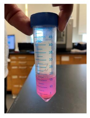
Sample immersed in SBF solution for 7 days
