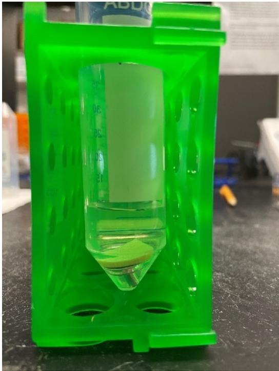
Sample immersed in SBF solution for 7 days
