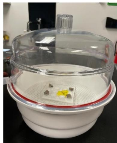
Samples placed in the vacuum desiccator
