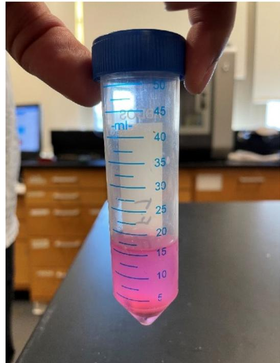
Sample immersed in SBF+DMEM solution for 7 days
