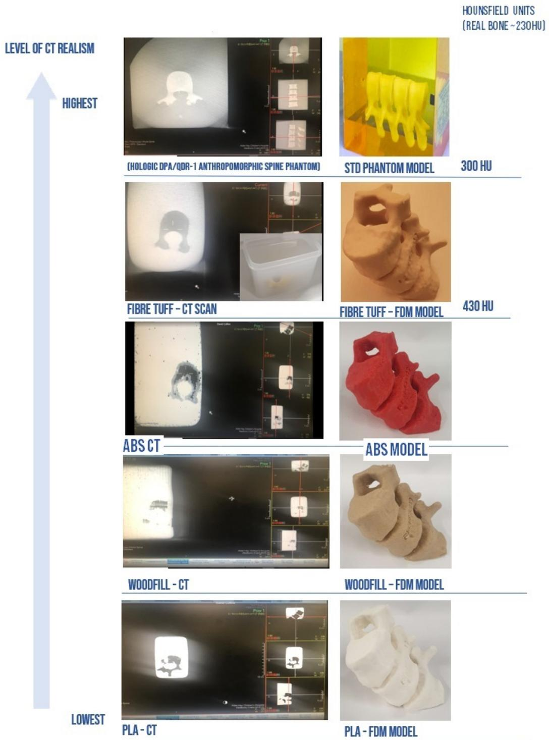
3D Printed Vertebrae made with FibreTuff on a Ultimaker 3 by 3D Lifeprints and CT scanned
