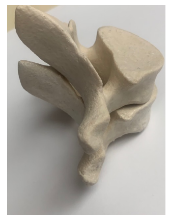
SLS printed vertebrae made with eco friendly coating
