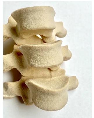
SLS printed vertebrae made without coating
