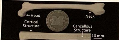
An X-ray computed tomography (CT)-based, biocompatible femur bone prototype, fabricated using FDM process at Marshall University.
