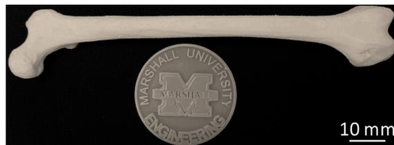
Figure 1: A 3D-printed bone, composed of Polyamide, Polyolefin and Cellulose fiber (FibreTuff, Perrysburg, OH), fabricated at Marshall University's Lab for Advanced Manufacturing and Engineering Systems (LAMES).
