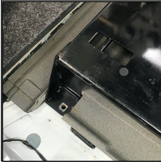
Passenger side (Inside-Rear) bracket with the cut rubber mat
