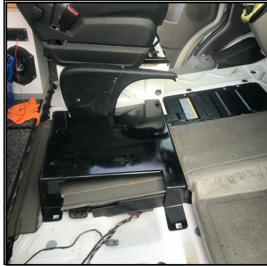
Showing the placement of the Base with the rubber mat re-installed
