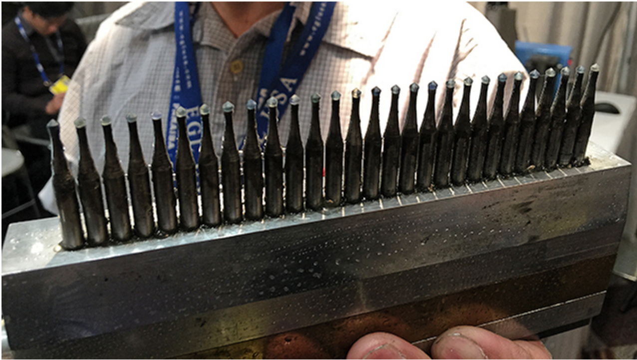
Figure 3. A cassette of stones is cut using water as a cooling agent. Photo by Tao Hsu.
