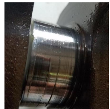
A "scarred" Triumph crankshaft
