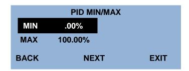
PID MIN/MAX – Sets the minimum and maximum the analog outputs can be ran at.
