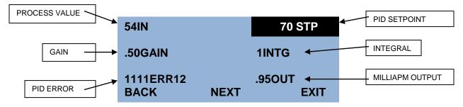
Gain – Speed of response. The higher the gain value, the slower the response.
