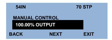
Use this screen to manually change the analog output to the VFD, Valve, etc.
