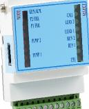
The PC102-S is similar to the PC101-S with additional monitoring functions for hand/off/auto selector position and critical alarm inputs such as pump overtemperature, VFD fault, etc.
