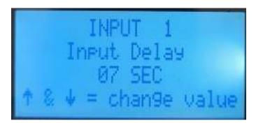
Use the up and down keys to set the delay time between the input activating and the channel alarming.
