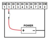
The common is negative. When positive is applied to the input, the indicator on the main screen will darken.
