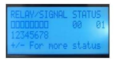
This screen shows the state of the relay outputs. An unfilled block □ indicates a deenergized relay. A filled block ■ indicates an energized relay.
