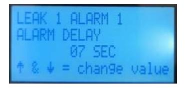
This will set the time delay before a text is sent out for a seal leak alarm.
