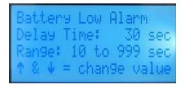
This screen sets the delay before the CM18 will text you when the battery is low.
