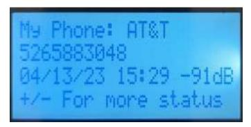
Starting with the top line, we show the cell carrier being used by the CM18, followed by the units phone number. The third line includes the date & time, which is updated from the cell towers. The cell signal strength, measured in db, is also shown on this line.
