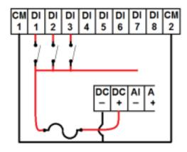
This example uses the 24VDC input terminals to drive the dry contacts from the field.
