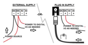
1 AMP at 24VDC is suggested for an external power supply. Our plug in supply is available when ordering.
