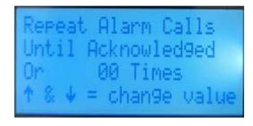
This screen sets the functionally of repeat alarm calls. Defaulted to 0, sets the amount of times the phone number list is texted for an alarm.
