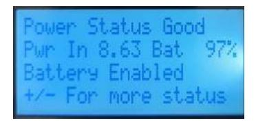
The second line shows incoming power of the CM18 along with the battery level in %. The third line shows the status of the battery.
