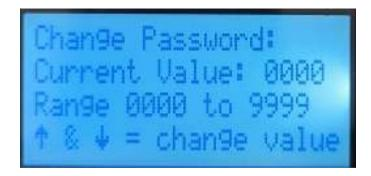
Defaulted at 0, the password can be changed at this screen. If changed, you must make note of this.
