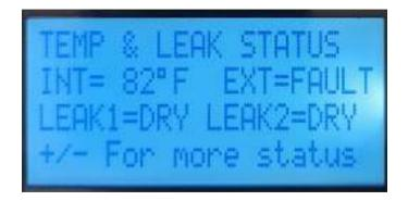
The second line on the screen shows the internal temperature of the CM18, along with a temperature reading of an external temperature connection.
