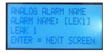
This screen views the current name of the seal leak alarms. Change it by texting the CM18 LEK1=
