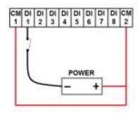
The common is positive. When negative is applied to the input, the indicator on the main screen will darken.
