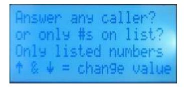
This setting will lock out any phone number that isn't in the recipient list from communicating with the CM18. It is highly recommended that this setting be changed to allow anyone to text the CM18 when setting up yours for the first time.
