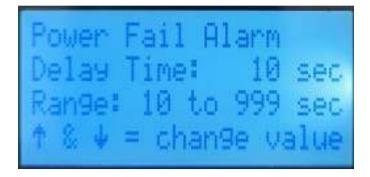
This screen sets the amount of time the CM18 will be without its main power source before going into an alarm.
