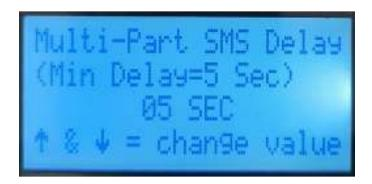
Defaulted at 5 seconds. This sets the delay between texts in a two part text. Press enter to go to the next screen.
