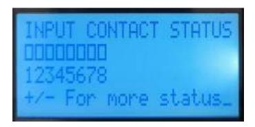
This screen shows the state of the digital inputs. An unfilled block □ indicates an open input, a filled block ■ indicates a closed input.
