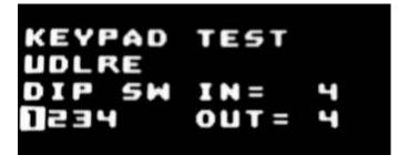
The next diagnostic screen shows the pushbuttons to troubleshoot the keypad. The DIP switches are read and shown. A block on the number indicates an ON state.
