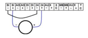
Connecting the RS485 Modbus® data. The ground is optional.
