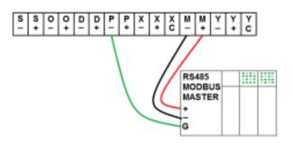
Connecting a Sigma Controls submersible sensor. The shield wire should be connected to earth ground. (Power should be fused)
