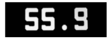
Pressing the Up key from the main screen will display the process value only. This large display allows the value to be seen from a distance.
