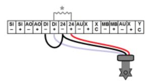
Connecting any 4-20mA, non-powered sensor.
