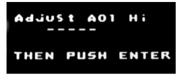
Adjust the up and down keys until the DVM reads 20.00mA then push enter.
