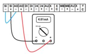
If you are using the default settings of 4-20mA input and output, the EZ-C can be calibrated without a milliamp simulator. A simple digital volt meter (DVM) can be used. The wiring above shows the analog output being routed through a DVM set to read DC milliamps. The output is calibrated first, then used as a milliamp source, to calibrate the input.
