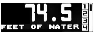
This is the screen that is displayed at the end of the power up sequence. The main process value is displayed with large numerals in the center of the screen. The engineering unit is displayed below the main process. On the far right a bar graph representing the range of the analog input. A heart symbol is shown beating, indicating a healthy processor.
