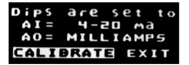
Again the user is encouraged to exit. The DIP settings are shown to ensure the proper calibration is performed. If you must change the factory set calibration, move the cursor to CALIBRATE and push enter.
