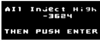
Inject 20.00mA. Push enter to save the new calibration.
