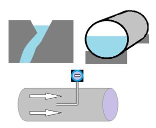
The linearizer is useful in applications where the analog signal needs to represent a round wall tank, weir or square root flow signal from a pitot tube.
