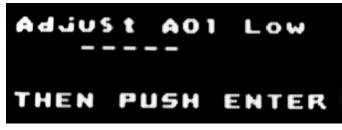
Adjust the up and down keys until the DVM reads 4.00mA then push enter.
