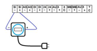
Connecting a powered 4-20mA or 0-10 volt signal.
