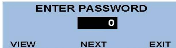
Enter the user selected password (factory default is zero) using the ↑ ↓ keys and press 'Enter' to access the first programming menu 'Menu 1'.
