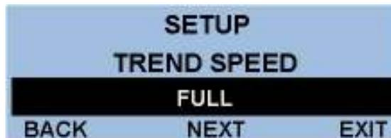
**NOTE:** The trend screen is provided as a diagnostic tool. This trend graphic will display the process value over the time duration selected. The duration of the trend is selectable between 2 minutes, 2 hours, 12 hours and full speed. The trend is non-retentive and will overwrite previous data.
