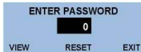
From the main menu press 'ENTER' key to access the 'ENTER PASSWORD' screen. Use the → ← keys to scroll to the 'VIEW' position and press 'ENTER'.
