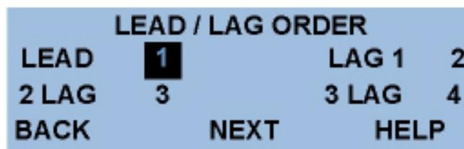
The example shows the #1 pump as the 'Lead', #2 as the 'Lag', and #3 pump as the second 'Lag'. The starting position of any pump may be changed in this screen by positioning the cursor with the → ← buttons and selecting the desired pump sequence. **NOTE:** If alternation is enabled, the pump sequence will change based on time or pump cycle. If alternation is selected to be 'off' then pump sequence will be 'fixed' per the selected 'pump order'.
