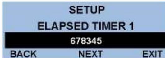
To reset the #1 timer use the ↑ ↓ keys to change the saved value to zero. Select 'NEXT' and press enter to access elapsed timer 2. Follow the procedure above to reset this timer to zero. Reset other timers in the same way.
