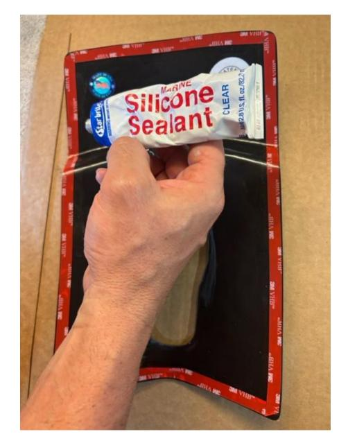
Apply a layer of marine silicone sealant (not provided) to the area (leaving 1  $\frac{1}{2}$ " of separation from the 3M double sided marine tape already installed on the part) as shown in the picture.
