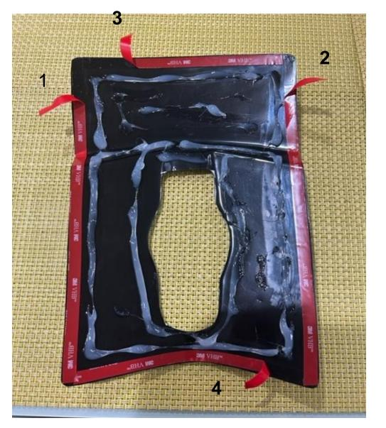
Now proceed to peel off the pre-cuts strips of 2" of each line of tape (as shown in the picture).
