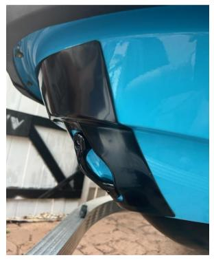
After install, please wait 72 hrs before going to the water so the adhesive can bond to the fullest according to the marine grade tape's manufacturing company and the marine silicone sealant used.
