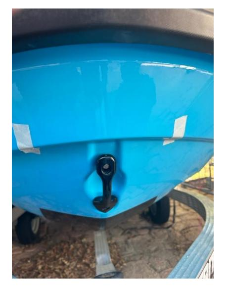
Once the part is positioned, mark the edges with masking tape (use 2" pieces) and 4-5" pieces to hold the part in place, as shown in the picture. Next, remove the part leaving just the masking tape as your guide
