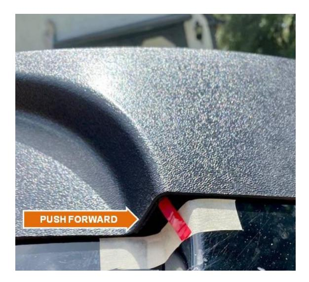
Once the part is aligned, push it forward at the bumps, so there is no room to move and make sure the ½" separation has been removed.
