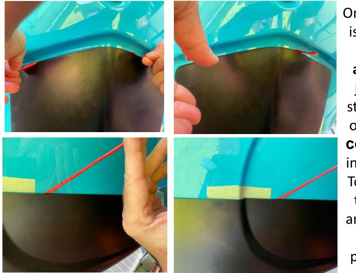
Once the part is fitted and there is absolutely NO GAPS, start peeling off the tape completely in this order: Top, Bottom then sides and carefully apply pressure all over
