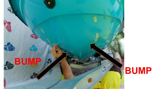
Proceed to finally attach the part using the **"BUMPS**" on the side of the hull of the wave runner as **your guide** to properly fit the part, **without applying any pressure**.
