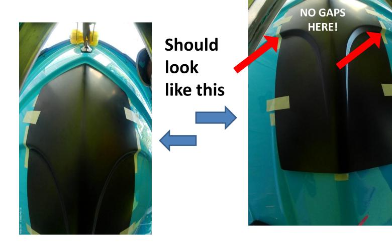
Next, remove the part leaving just the masking tape as your guide.
