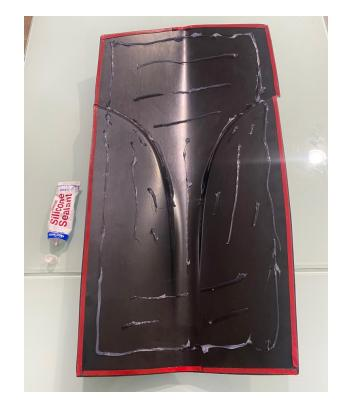
Once the part is completely clean, apply a layer of marine silicone sealant (not provided) to the area (leaving  $1 \frac{1}{2}$ " of separation from the 3M double sided marine tape already installed on the part) as shown on the picture.
