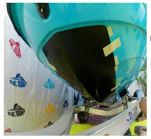
Once the part is positioned, mark the edges with masking tape (use 2" pieces) and 4-5" pieces to hold the part in place, as shown in the pictures)
