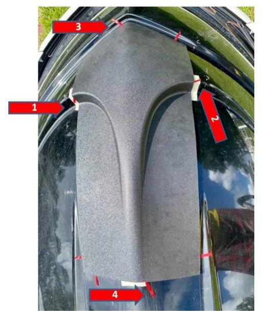
Make sure the peeled off strips of tape are not under the part but outside.
