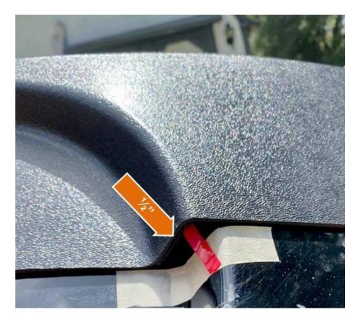
First, position the part ½" away from the BUMPS (as shown in this picture). The idea is not to attach it completely yet.
