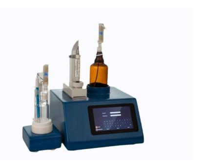
K. F. is a titration process used to calculate the moisture % of sample using a known standard. IRIS Software Provides a Sophisticated Report generation process with ease of reading.
