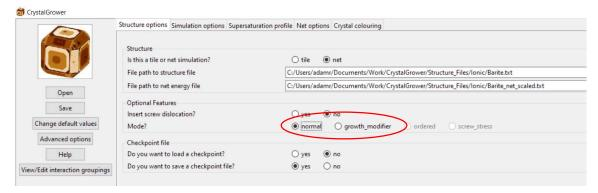
"growth\_modifier" simulations are to be used in situations where molecular impostors / poisoning agents / growth modifiers are added to a solution of crystallising material. An additional tab is created for controlling the behaviour of the growth modifier. Please consult the detailed growth modifier section of the manual for more information.
