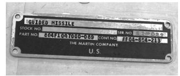
Nameplate on underside of aft skirt. approximately .050 inches (1.27 mm) to .170 inches (4.3 mm) depending on the location. For comparison, a U.S. dime is .053 inches (1.35mm) thick, while a quarter is .068 inches (1.75 mm). Chemical milling was used extensively to reduce the thickness, and hence the weight, of the airframe. Titan II's weight, including the reentery vehicle (RV) and propellant, was nominally 330,000 pounds (150,000 kg)—a number made even more impressive when
