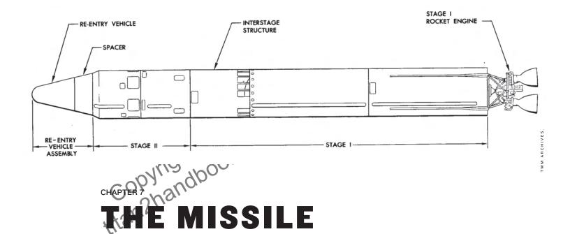
Standing 103 feet (33.5 m) tall, with a range of over 6000 miles and topped with the largest thermonuclear bomb ever carried by a U.S. ICBM, Titan II was the blockbuster of the United States' nuclear deterrent. The main body of the missile, often referred to as the *airframe*, was 10 feet (3 m) in diameter and constructed from anodized aluminum, alloy
