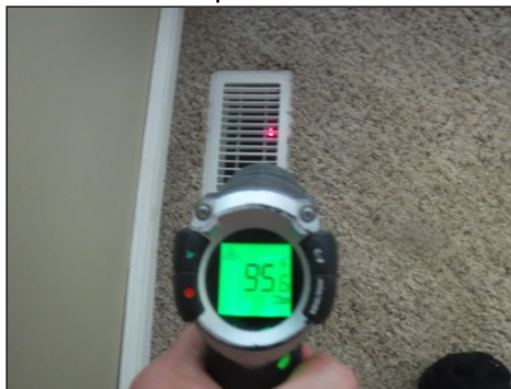
Heating air temperature during operation (95 degrees)
