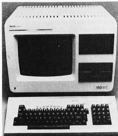
Motorola 68000, 256K memory, 10MB Winchester disk, 760KB floppy, terminal, system software, choice of Pascal, FORTRAN, C, Assembler, BASIC, COBOL
