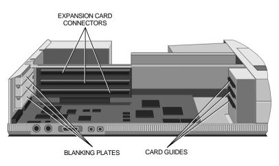
At the rear of the area are three metal blanking plates, one for each expansion card slot. These plates cover slots in the rear of the system unit which will be used by expansion cards.
