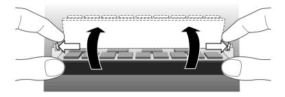
3. When the SIMM has rotated through 20°, taking care to avoid touching any of the components on the SIMM, grip the top corners of the SIMM between thumb and first finger and carefully pull the SIMM out of the socket.
