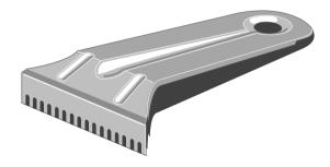
5. Carefully insert the prongs of the extractor between the bottom of the processor and its socket. You may need to twist the extractor gently from side to side to work the prongs into place.
