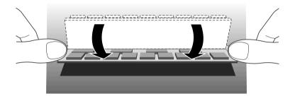
5. If the SIMM is properly located the SIMM should remain in position held by the securing clips, and with a small plastic lug through the holes on either side of the SIMM.
