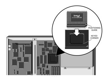
2. Carefully position the upgrade processor above the socket with the positioning guide on the processor over the keyed corner of the socket.
