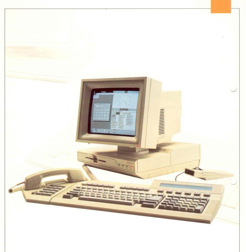
Apricot XEN-i combines the performance of Apricot XEN with full IBM® compatibility. It is capable of processing speeds 30% faster than its competitors, with an Intel™ 80286 processor running at 10 MHz. It retains the elegant style and small footprint which are
