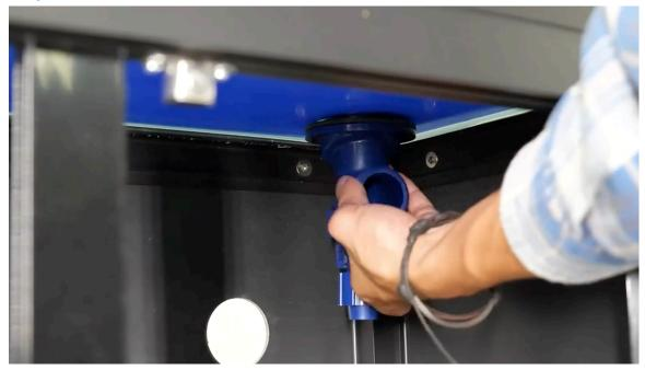
Screw together and tighten the bottom half (A) and top half (B) of the plumbing bulkhead — hand-tight only.
