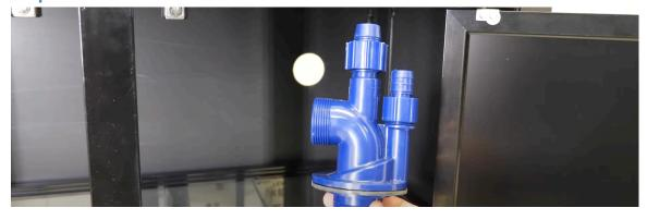
Take the bottom half of the plumbing bulkhead (A) and align it through the hole to the top half (B).
