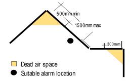
If a flat or sloping ceiling has closely spaced exposed beams the areas in between the beams should be considered as dead air space and the alarm should be attached to the bottom of a beam.
